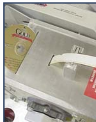
Small destruction slot accepts key tape strips or rolls. Large slot is for optical media.
